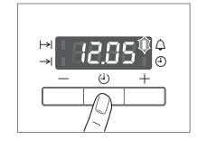
2. Using the + or — button set the desired Countdown (max. 2 hours 30 minutes).
